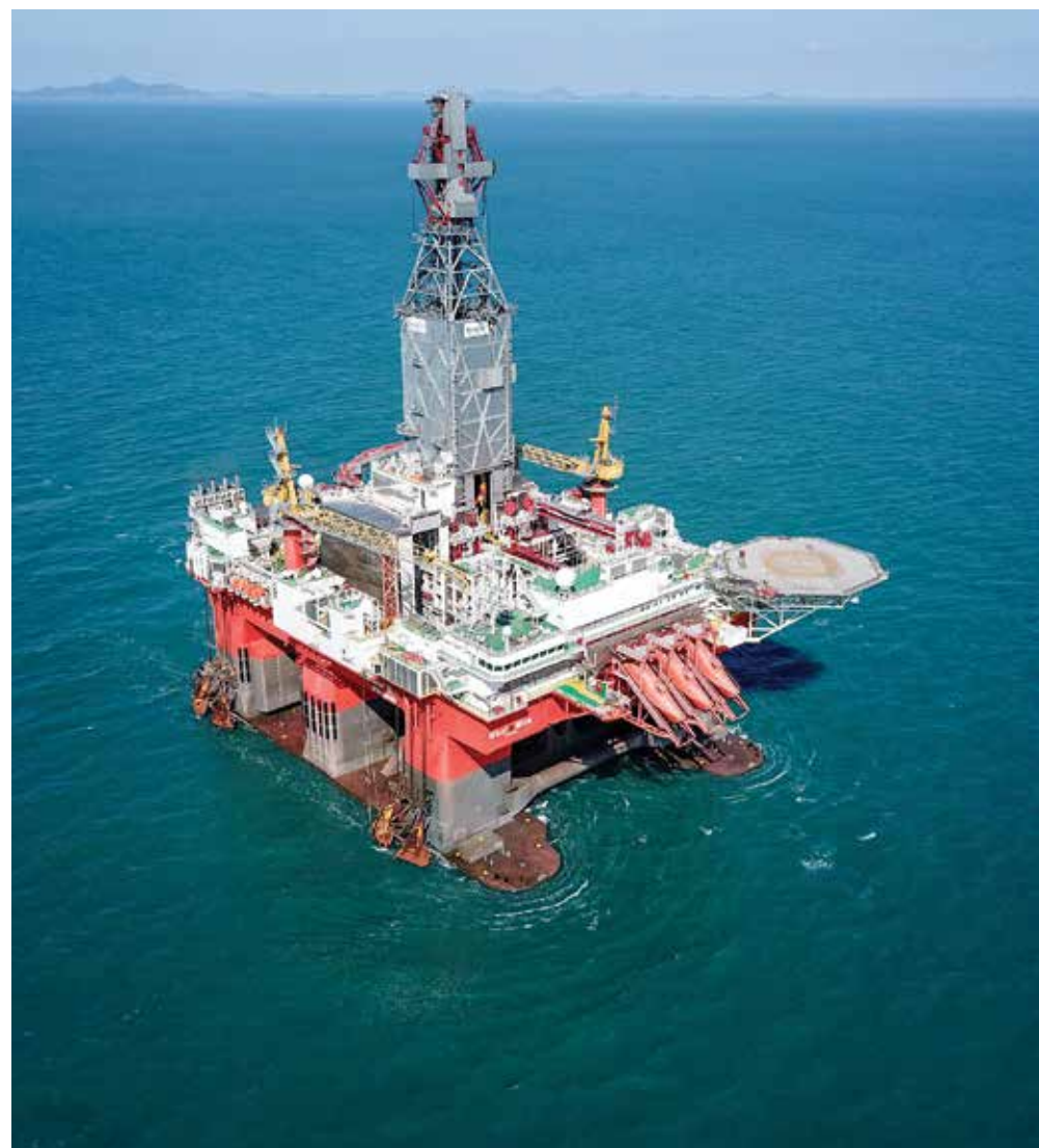
FIG. 1. West Mira will operate on a low-emission plant powered by lithium-ion energy storage. Photo copyright: Neil Robertson
