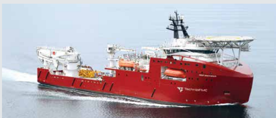
The 121-m-long Deep Discoverer can cruise at 14 knots and features an 18-person, twin-bell, 300-m diving system. Image: TechnipFMC.
